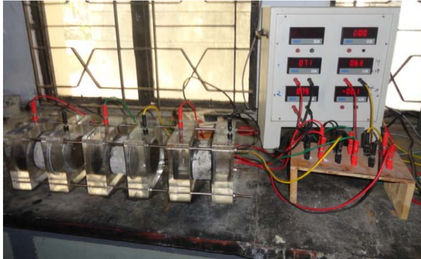
Figure 4.3: Photograph of RCPT setup
