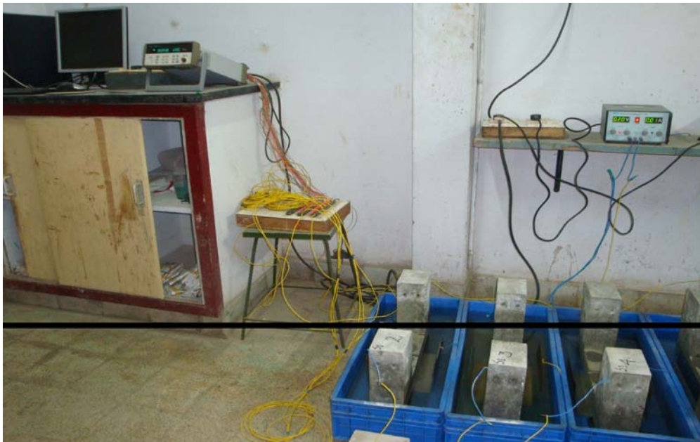
Figure 4.4b: Typical view of accelerated corrosion test set-up with data-logger: Uncracked specimens without tie rods (closer view)
