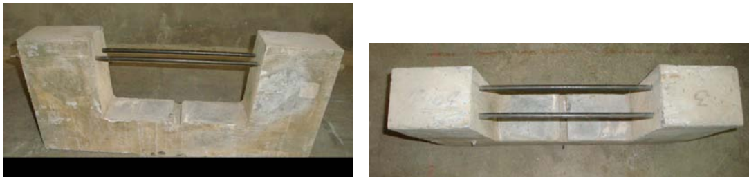
Figure 3.3: Cast specimen with tie rods
