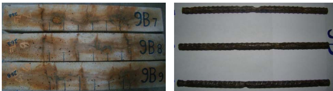
(c) 0.4 mm crack width specimens
