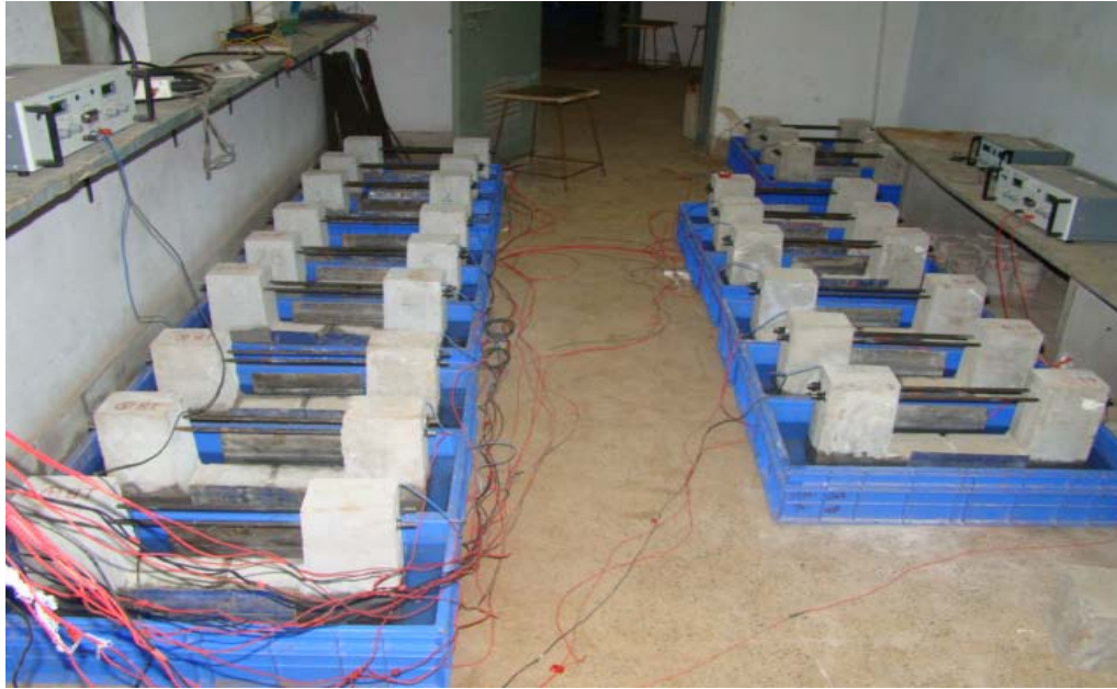
Figure 4.5: Typical view of accelerated corrosion test set-up: Cracked specimens with tie rods
