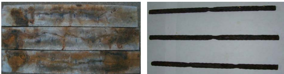
0.4 mm crack width specimens
